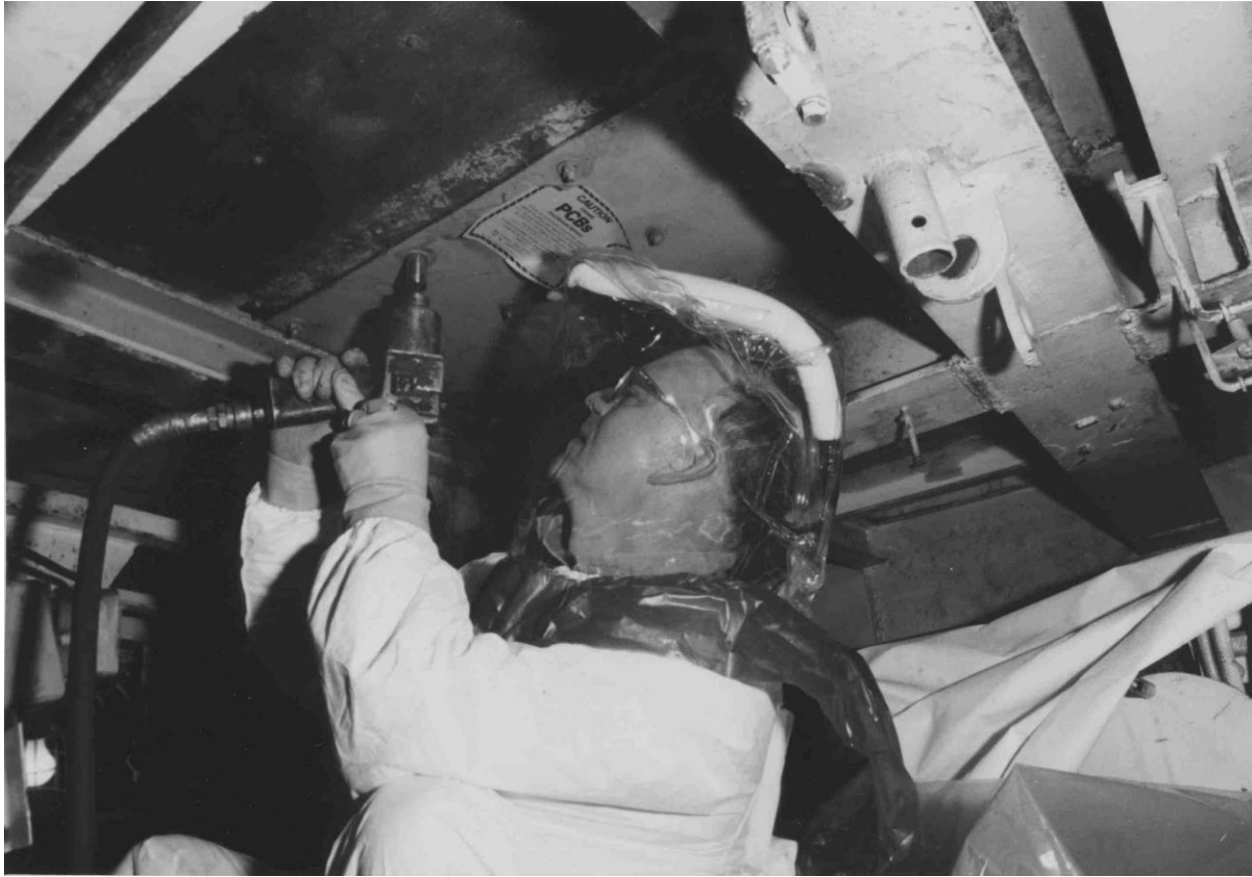
Shipboard Removal of Cover Plates to Allow Access to Remove PCB Felt Sound Damping Material
