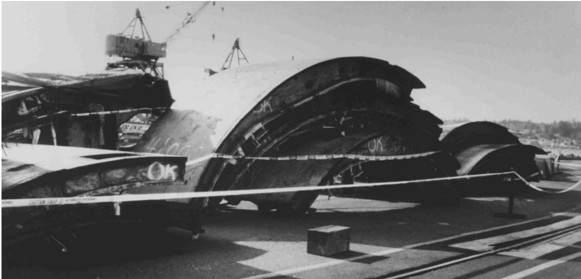
Staged Submarine Hull Sections
